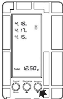
Connect the battery on the right side balancer jacks so that the display is activated.
