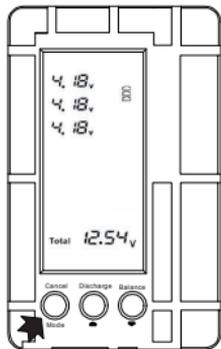
For the first use the minimum discharge- and balancer voltage must be checked and adjusted if necessary. For this connect a battery to the balancer connector on the side so that the display is activated.
