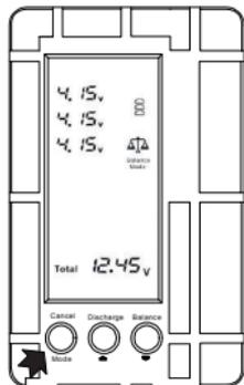
3. The balance process is complete when all scale icons are off. Now press the button „Cancel“ to exit. You can now disconnect the battery.
