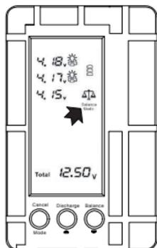
2. The balancer accepts the lowest cell voltage as a reference and starts the balancing process indicated by the scale icon. The flashing scale icon appears behind these cells which are currently balanced active.
