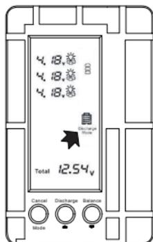
2. The balancer starts the balancing process indicated by the battery icon. The flashing
