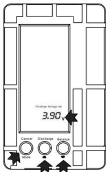
3. „Mode“ button is pressed twice: Setting the discharge voltage limit. *Attention: check the minimum storage voltage of the connected battery type!*
